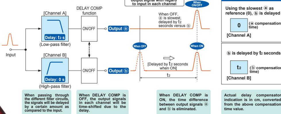
When a signal passes a filter circuit, a delay necessarily occurs. The "DELAY COMP" function compensates for such delays. The illustration at left uses a 2-way system as an example to show how the delay compensator works.
