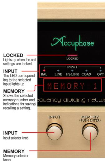
Turn the INPUT knob to select an input (respective LED lights up).
