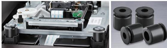
Traverse mechanism supported by viscous dampers
